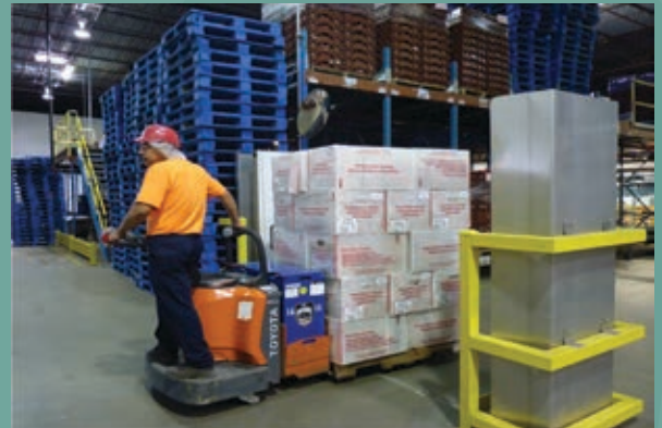
25 Full boxes pass thru RFID portals on their way to distribution
