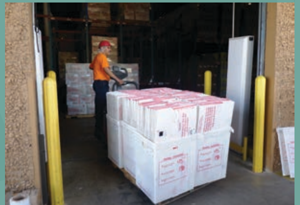
Knocked down and utilized in master return tubs, 150 boxes pass thru RFID portals returning from distribution
