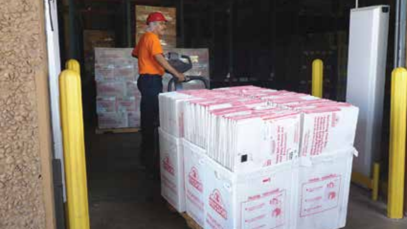
Knocked Down and Unitized in Master Return Tubs, 150 Boxes Pass Thru RFID Portals Returning from Distribution
